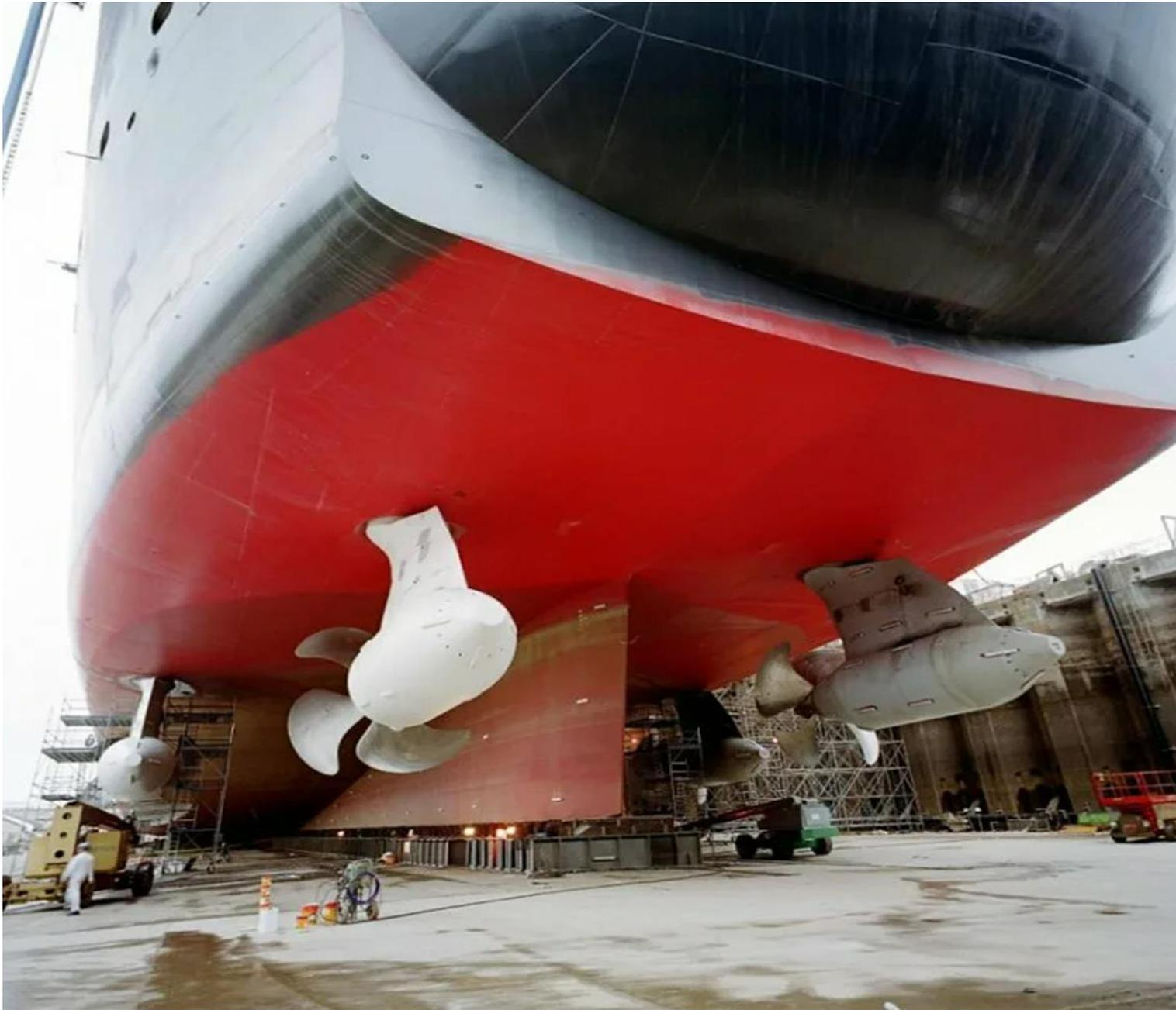
Queen Mary 2 features four Mermaid pods built by Rolls Royce-owned Kamewa and Alstom Powers Motors. She is the first passenger ship to be driven by four pods. **The forward two pods are fixed in place** while the aft two are able to turn through 360degrees to steer and manoeuvre the ship.
