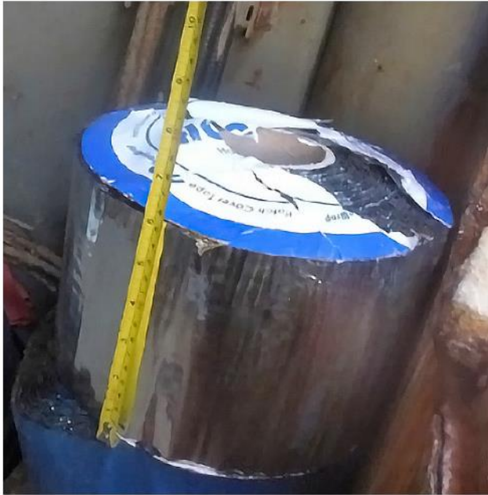
Figure 16: Hatch cover sealing tape
